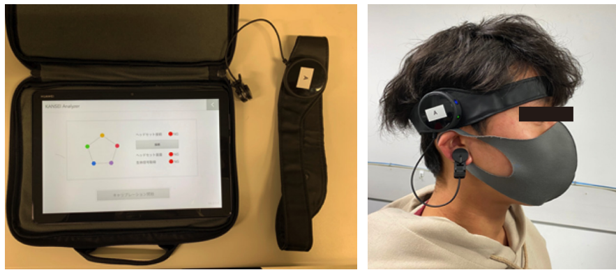
Fig. 1 Kansei analyzer (left: components; right: application on a subject).
